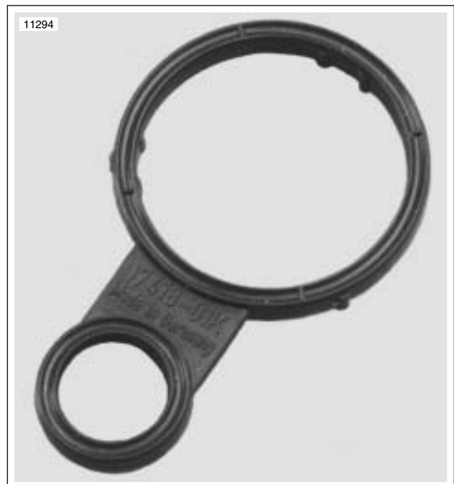
Figure 1-92. Spark Plug Hole Gasket (double lipped side)
