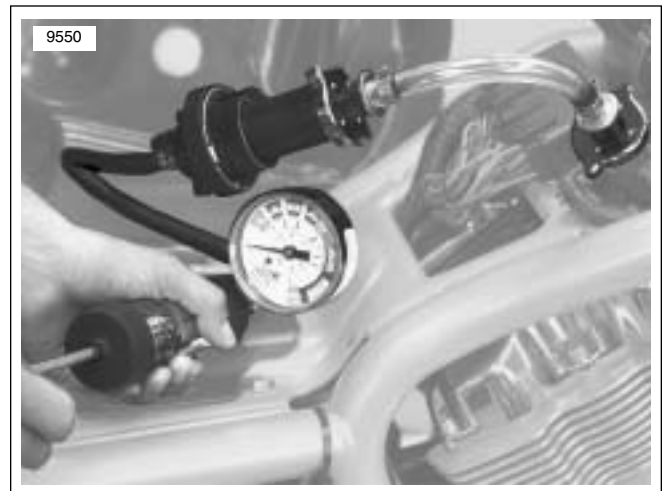
Figure 6-5. System Pressure Test
