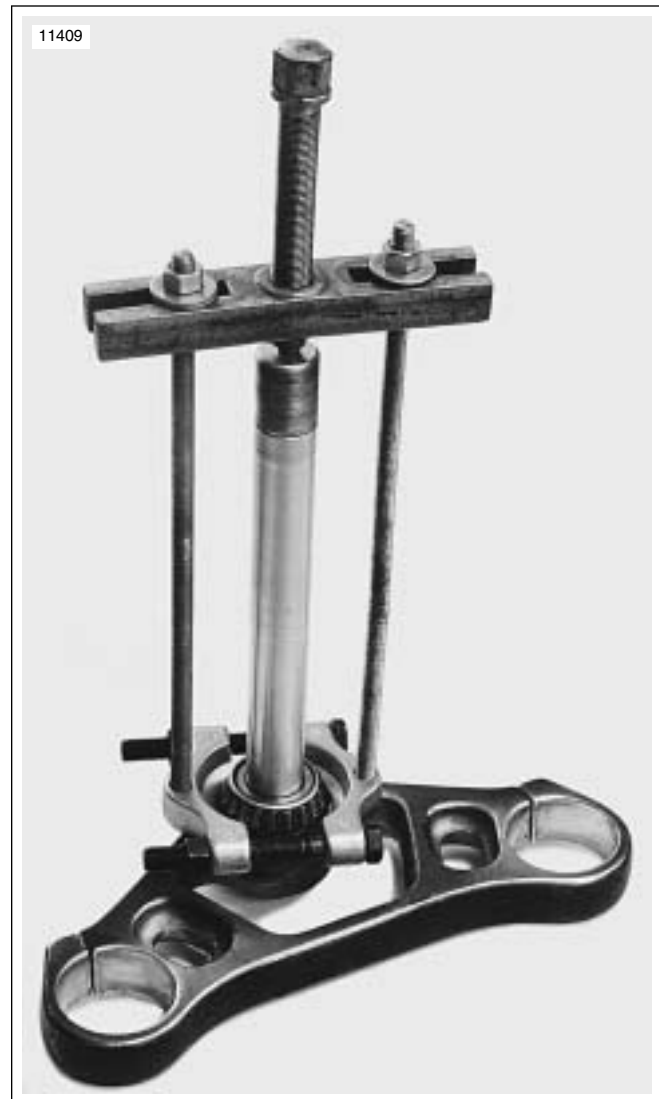
Figure 2-149. Bearing Puller Based on Universal Wedge Attachment (typical) (VRSCA shown)
