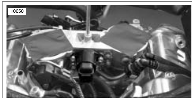
Figure 8-17. Airbox Removed, Injector Intakes Protected
