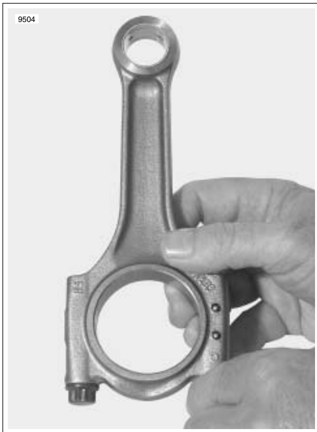
Figure 3-206. Install Rod Caps For Inspection
