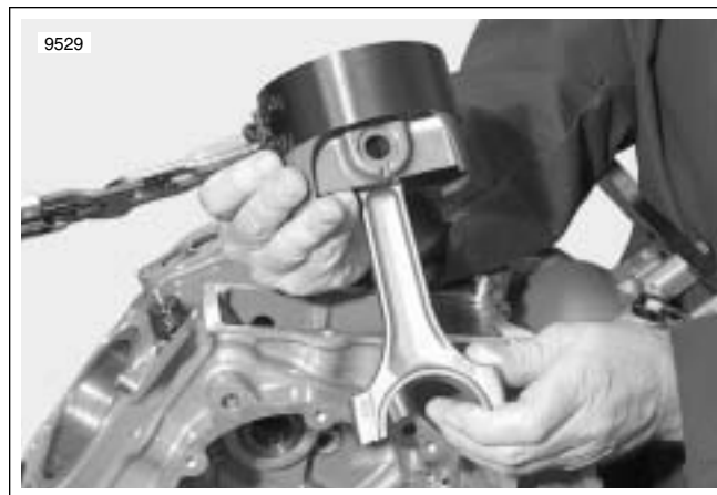
Figure 3-226. Piston Ring Compressor
