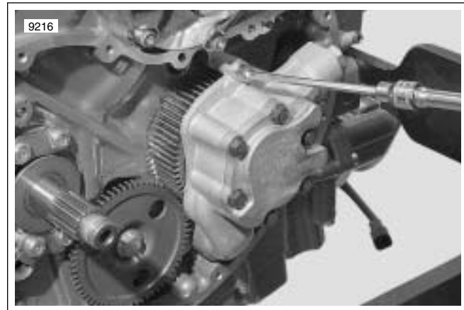
Figure 3-65. Remove Oil Pump
