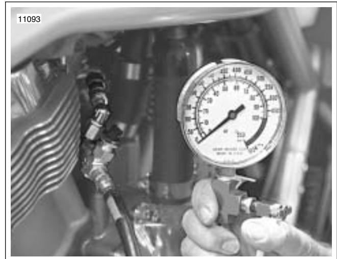
Figure 4-50. Fuel Pressure Gauge Installed
