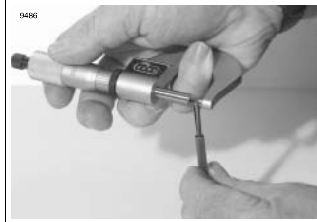
Figure 3-52. Measure Stem to Guide Clearance
