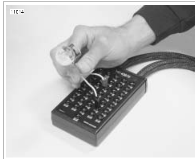
Figure 8-84. Ignition Coil Circuit Test
