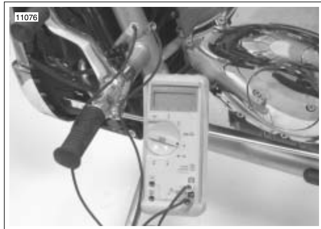
Figure 1-19. Check for Stator Resistance (typical)
