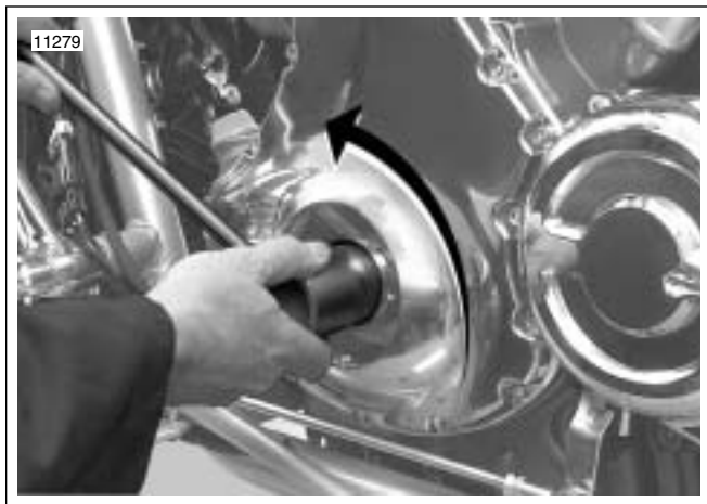
Figure 1-73. Correct Engine Rotation
