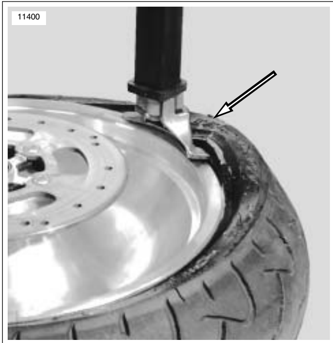
Figure 2-93. Tire Machine Pulling Bead Off Rim
