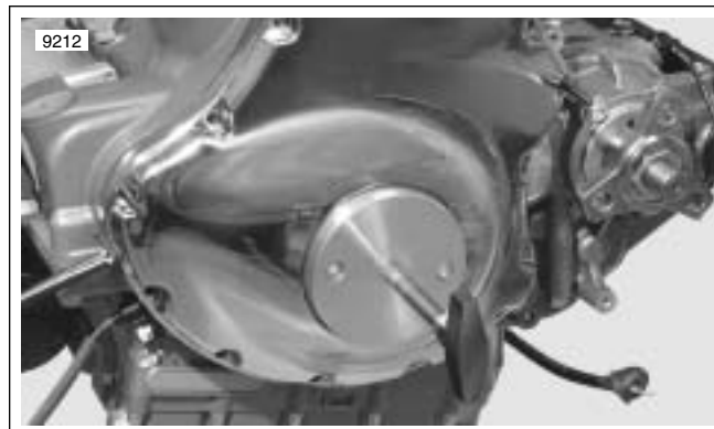
Figure 3-108. Position Tool HD-45304
