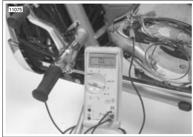
Figure 1-18. Test for Grounded Stator (typical)
