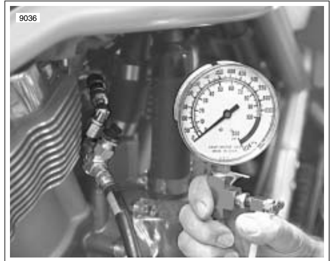
Figure 4-44. Fuel Pressure Gauge Installed
