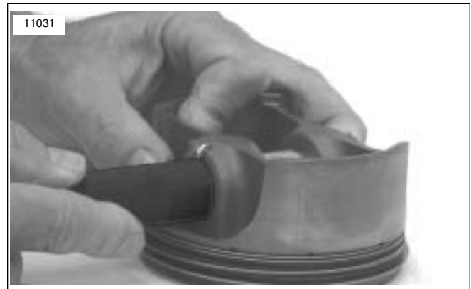
Figure 3-3. Piston Pin Clip Installed and Seated
