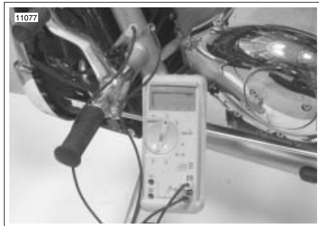
Figure 1-20. Check Stator AC Voltage Output (typical)
