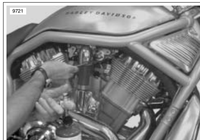
Figure 4-46. Checking for Leaks (typical) (VRSCA shown)
