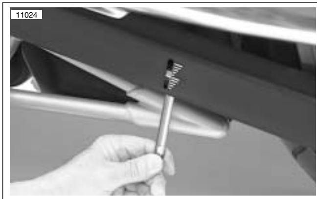
Figure 2-22. Determining Belt Deflection Using OEM Belt-guard and Belt tension Gauge (HD-35381))
