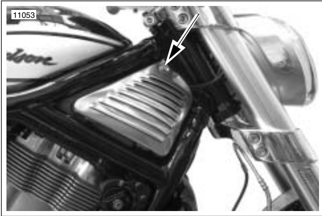
Figure 1-16. Removing Fastener and Cover to Check Coolant Level (typical)
