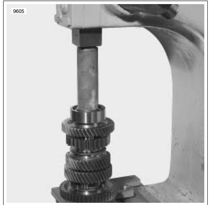
Figure 7-8. Output Shaft Bearing
