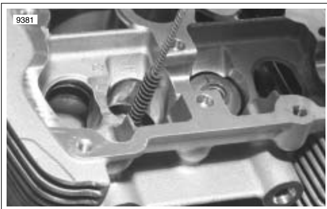
Figure 3-50. Hone Valve Guide
