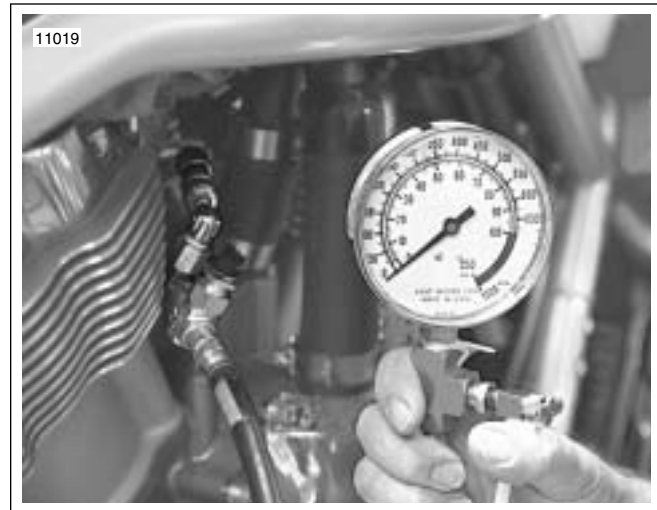
Figure 8-104. Fuel Pressure Gauge Installed
