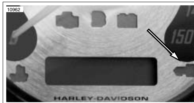
Figure 8-40. TSSM Lamp Location
