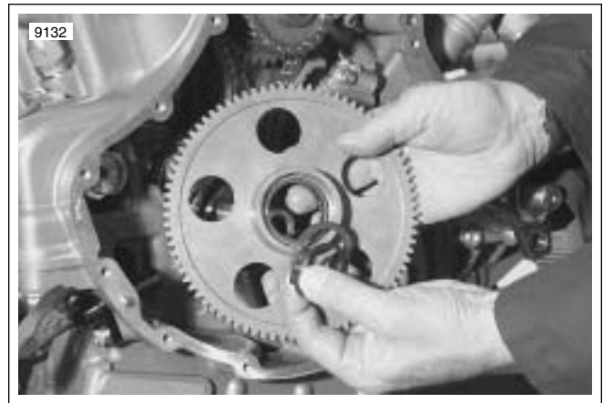
Figure 3-274. Needle Roller Bearing, Ball Gear, Thrust Washer and Retaining Ring
