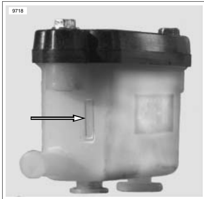
Figure 2-60. Rear Brake Reservoir Sight Window (removed from motorcycle)
