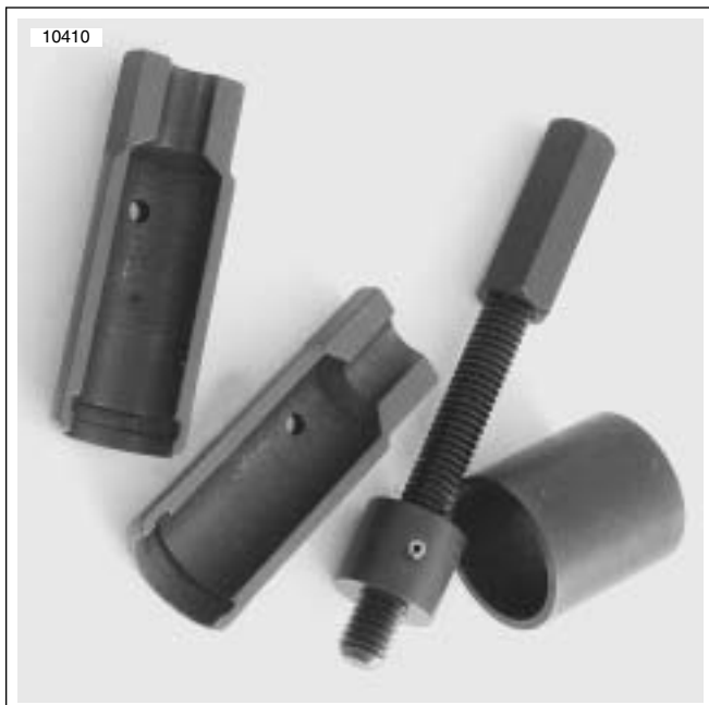
Figure 3-165. Counterbalancer Bearing Inner Race Remover and Installer (HD-46582)
