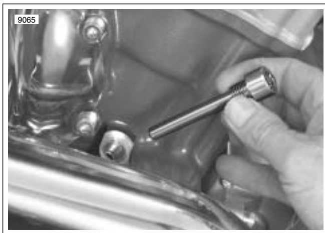
Figure 3-140. Crankshaft Locking Pin (HD-45306)
