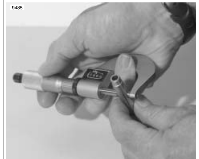
Figure 3-47. Valve Guide Dimensions
