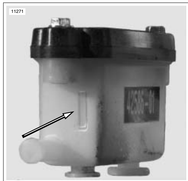
Figure 1-31. Rear Brake Fluid Reservoir Sight Gauge (reservoir removed from motorcycle) (typical)
