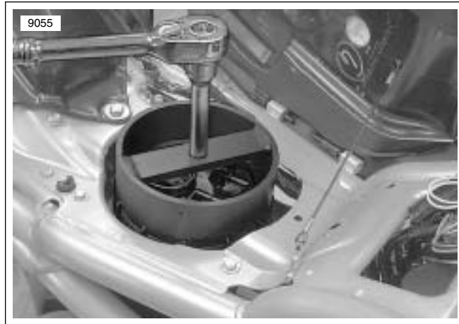
Figure 4-3. Fuel Cap Remover/Installer (HD-45324)
