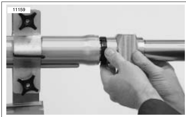
Figure 2-132. Install Bushing, Spacer, and Install Fork Seal in Place with Seal Driver (B-45305)
