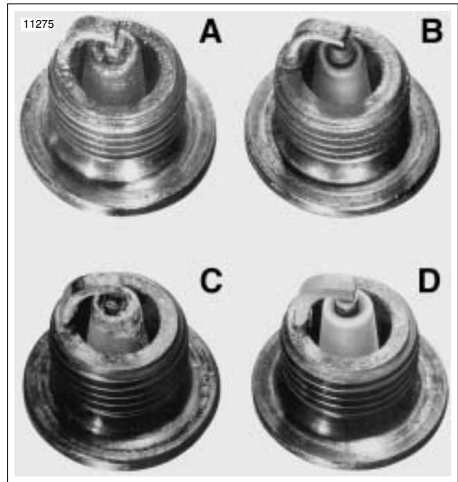
Figure 1-62. Typical Spark Plug Deposits
