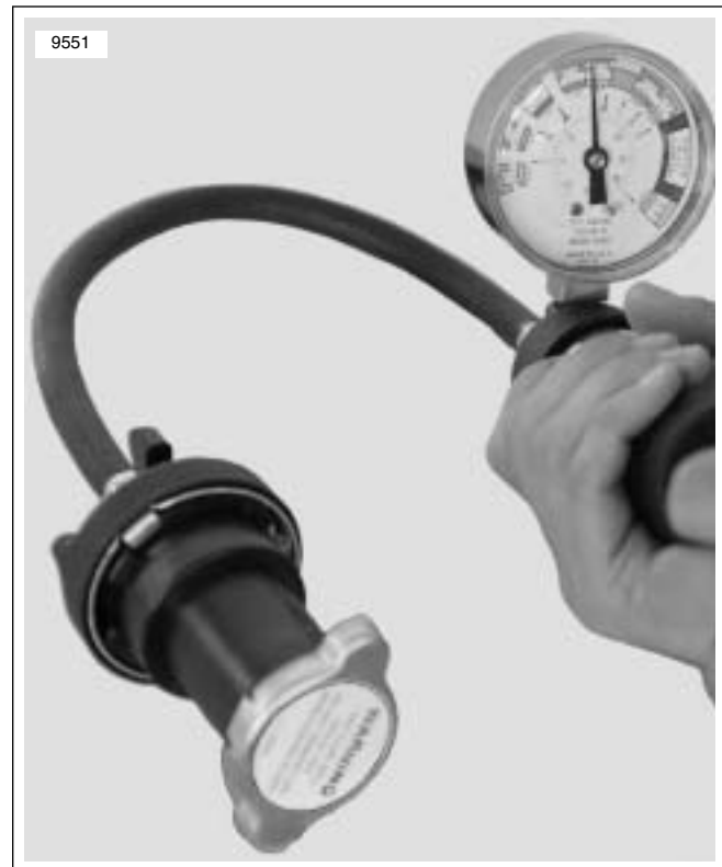
Figure 6-4. Pressure Cap Test
